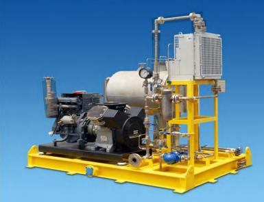
A customized Marine Startup Air Compressor package for P53 Petrobras FPU Conversion Project
